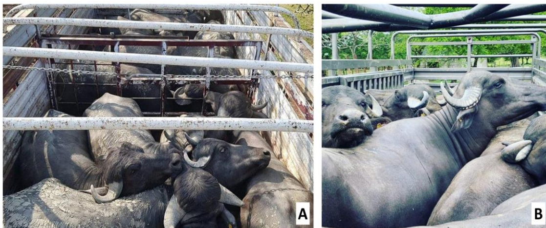
Figure 3 Physical adaptations of vehicles used to transport water buffaloes. A. A truck with the recommended load density reduces the risk of falls and injuries due to the space provided per animal. It is equipped with physical divisions to transport animals of different ages, sizes, or origins. B. Vehicles with a roof design provide ventilation but do not open any means of escape.
