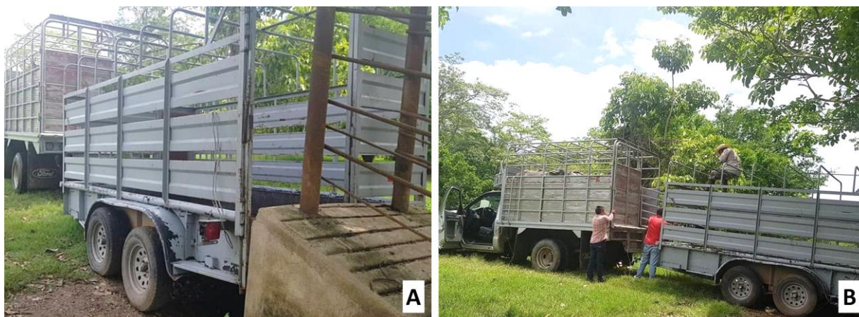
Figure 7 Loading and unloading ramps used in Mexico for buffalo transport. A. Trailer and uneven ramp. Though it has slots and an adequate slope, this ramp is not aligned correctly with the trailer, a factor that may cause injuries to the buffaloes' hind limbs. B. Type of trailers used to transport buffaloes in Mexico.
